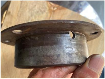
Far left is the rear bearing housing showing half round slots filed into the rim to aid future removal. Left is the side view showing the oil feed hole to the bearing, very important to line this up with the hole in the crankcase.
