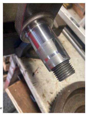
The 'shrunk' front axle arrived next, and I wasted no time getting it back on the chassis. I now have very nice tight king-pin holes, ready to take the stub axles. I had ordered new bushes for the original semi-Girling stub axles, and have fitted them. However, they will need reaming with a ½ " reamer.
