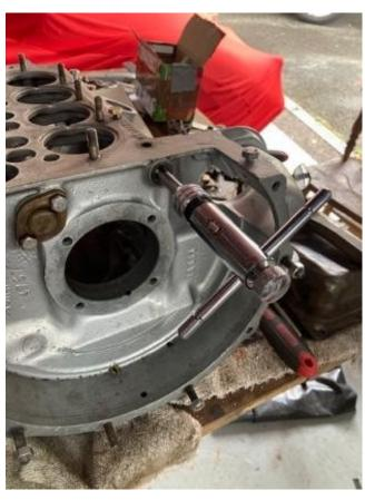
Before starting this work, I read through the excellent article written by Bob Garrett on engine rebuilds. I must have read it five times. One thing Bob suggests, as do others, is the introduction of an external full-flow oil filter, as the filter on the original engine is only a mesh screen in the sump. Bob explains very clearly how this is to be done by tapping the main oil gallery in the crankcase.
